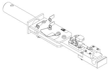
Model: 01-0812-0000 Bombardier CS100/300 Towbar Head
