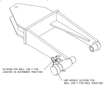
FIGURE 6 - Sliding Pin Position for Starship
