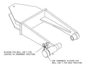
FIGURE 8 – Sliding Pin Position for King Air 90-B
