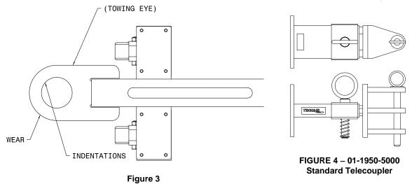
Tronair recommends a telecoupler pintle hook arrangement. This arrangement is known to eliminate binding. Tronair offers a Standard Telecoupler, Model Number 01-1950-5000, for use on tugs. *Reference Figure 4.*
