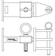
FIGURE 3 01-1950-5000 Standard Telecoupler
