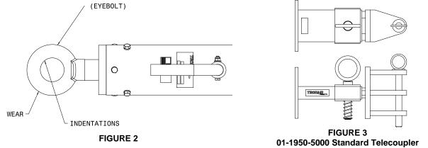
Tronair recommends a telecoupler pintle hook arrangement. This arrangement is known to eliminate binding. Tronair offers a Standard Telecoupler, Model Number 01-1950-5000, for use on tugs. *Reference Figure 3*.
