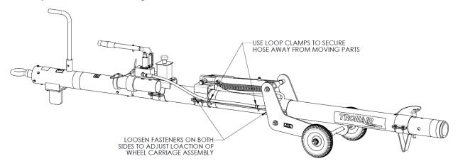
Alternatively, the landing gear assembly may be flipped to improve downward force at the head end of the towbar. Remove the hydraulic hose from the loop clamps, and remove the fastening hardware from both sides – 8 places total. Rotate the towbar or lift assembly 180° and reinstall. Adjust and relocate the loop clamps as needed to restrain the hydraulic hose.
