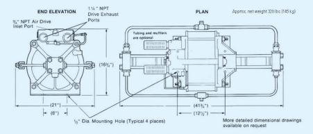
Note: See 29079 interconnecting tubing optional page 15. (29079 shown) Single Inlet port – % JIC male flare connection, single outlet port % HP ports (BuTech). Individual Pump ports – Liquid inlets 2 ea. ½ NPT ports, 2 ea. % HP ports (BuTech)
