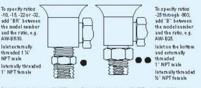
Drive inlet and exhaust are 1X\*NPT female. Drive inlet also includes a 1X\*NPT male x1X\*NP5M female (straight pipe thread) swivel adapter (connecting male nipple should include 30\*inside bevel for proper nit).
