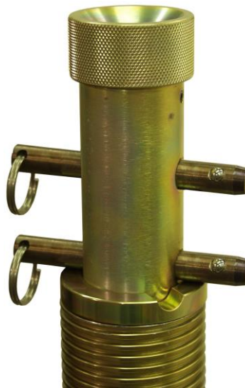
Locking Pin Not In Ram Protection Ring and top Locking Pin in Mechanical Extension (use only one pin)
