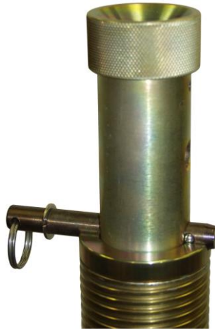
Ball Lock In Ram Protection Ring
