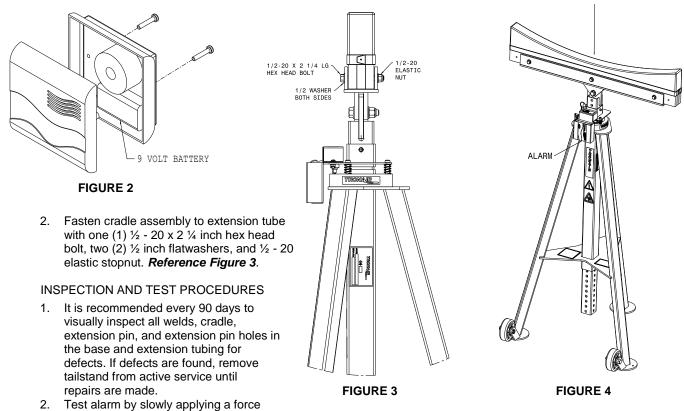
evenly distributed across the top of the cradle. The cradle head will lower and engage a limit switch. A loud pulsating alarm will then sound when the force reaches between 100 to 150 pounds (45.36 to 68.04 kg). If alarm does not sound, refer to the Troubleshooting section. *Reference Figure 4*.
