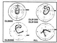
mum operating load requirement is 50 lbs. (23 kg) for Models DLB800, DLB800G, DLB1200 and DLB1200G, 75 lbs. (34 kg) for DLB1500 and DLB1500G, 175 lbs. (80 kg) for DLB2000 and DLB2000G.
