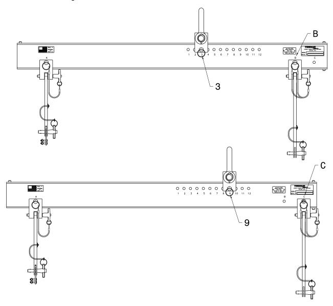
A rear lift plate is included with the engine sling. This will be removed and assembled to the engine with provided fasteners. See *Figure 2 – Page 2*.
