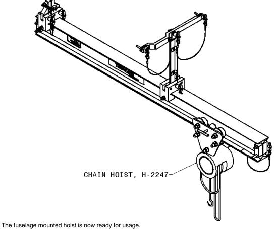
4. The fuselage mounted hoist is now ready for usage.5. To remove the fuselage hoist, reverse installation instructions.
