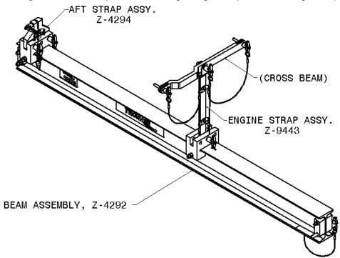
2. After the I beam is hung in place by the mounting straps, assembly the trolley on the I beam by pulling the front stop and rolling the trolley onto the I beam. After the trolley is installed onto the I beam, install the stop pin.
