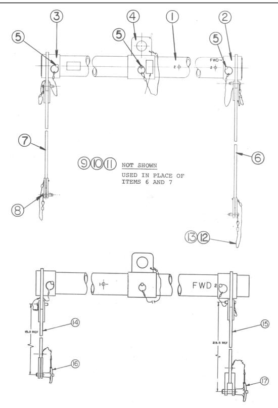
NOTE: Strap assemblies 14 and 15 are used to lift turbomachinery module. Lifting eye (Item 4) and sleeve assy-fwd (Item 2) are placed in position 2 when lifting turbo-machinery module.
