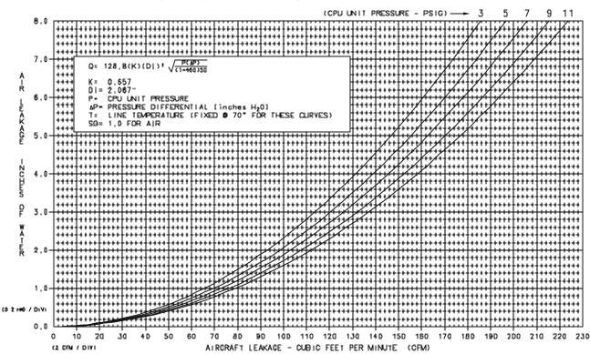
CURVE #2 PRESSURE COMPENSATED FLOW @ 70° F: INCHES OF H<sub>2</sub>O vs. LEAKAGE
