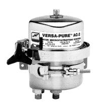
GENERAL ECOLOGY Versa-Pure™ AC-2 **Drinking Water Microfiltration System for** Aircraft - Designed for utmost reliability, maximum capacity per unit space and lowest pressure drop. Polished stainless steel, available with mounting bracket for coffeemaker and direct galley installations. Both SAE 37° JIC flare, and Mil Spec 33514 E6 flareless fittings (shown above) are available.
