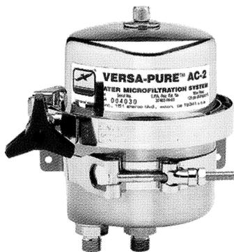
**GENERAL ECOLOGY Versa-Pure™ AC-2 Drinking Water Microfiltration System for Aircraft** - Designed for utmost reliability, maximum capacity per unit space and lowest pressure drop. Polished stainless steel, available with mounting bracket for coffeemaker and direct galley installations. Both SAE 37° JIC flare, and Mil Spec 33514 E6 flareless fittings (shown above) are available.
