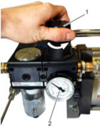
Fig. 18: Opening pressure regulator
