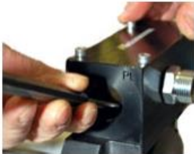
Fig. 39: Punching out the sleeve
