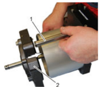
Fig. 78: Installing air pipes and lower cap
