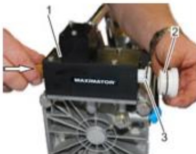
Fig. 30: Detaching spool valve and cap
