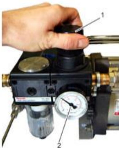
Fig. 23: Adjusting the operating pressure
