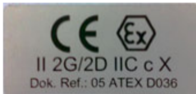
Fig. 94: Ex marking explosion group IIC
