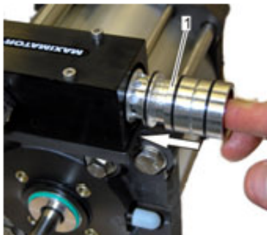
Fig. 42: Inserting the sleeve
