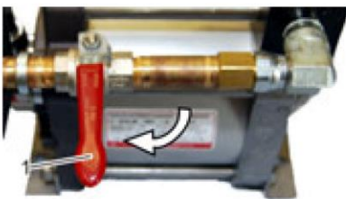
Fig. 26: Close ball valve
