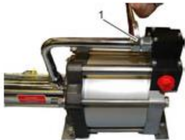
Fig. 83: Fastening the cooling pipe
