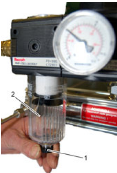
Fig. 25: Checking the water separator
