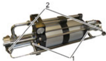
Fig. 53: Removing the cooling pipe
