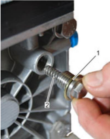
Fig. 51: Fastening the pilot valve
