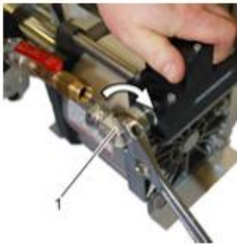
Fig. 36: Removing the elbow union
