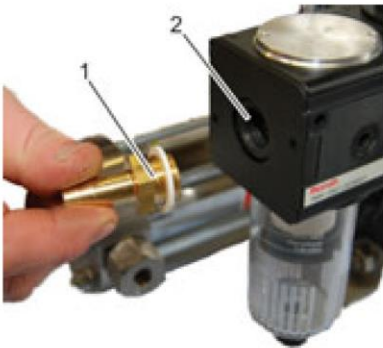
Fig. 10: Drive air connection (compressed air control unit)
