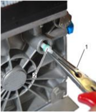
Fig. 48: Removing the pilot tappet
