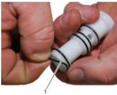
Fig. 32: Sliding on new O-rings
