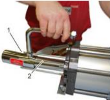
Fig. 82: Cooling pipe and high pressure pipe
