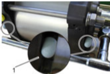
Fig. 12: Removing breather silencer
