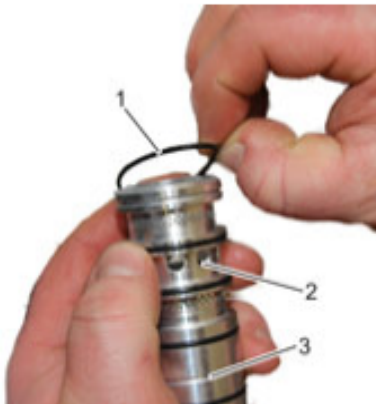
Fig. 41: Detaching the O-rings
