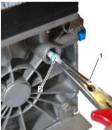
Fig. 50: Inserting the pilot valve tappet
