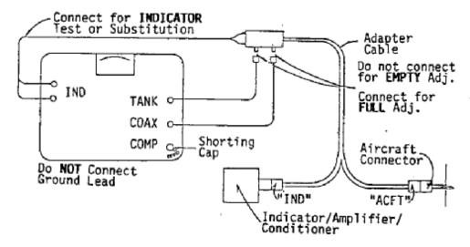
Figure 18 SYSTEM CALIBRATION (METHOD 1), CONFIGURATION #3 (BNC CONNECTORS)
