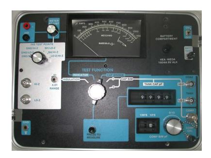
Figure 4 2548H FUEL QUANTITY TEST SET
