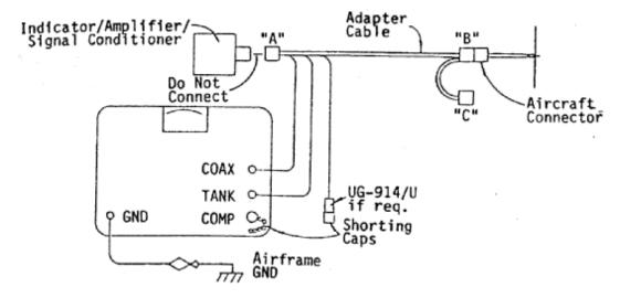
Figure 16 SYSTEM CALIBRATION (METHOD 1), CONFIGURATION #1 (MULTIPLE AIRCRAFT CONNECTORS)
