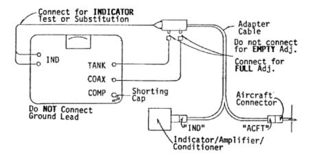
Figure 15 CAPACITANCE SIMULATION, CONFIGURATION #3
