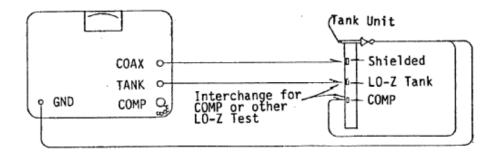
Figure 11 INDIVIDUAL TANK UNIT CAPACITANCE TEST, CONFIGURATION #1
