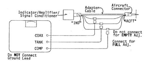
Figure 14 CAPACITANCE SIMULATION, CONFIGURATION #2
