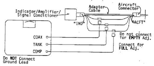
Figure 17 SYSTEM CALIBRATION (METHOD 1), CONFIGURATION #2 (SPLIT LEADS)
