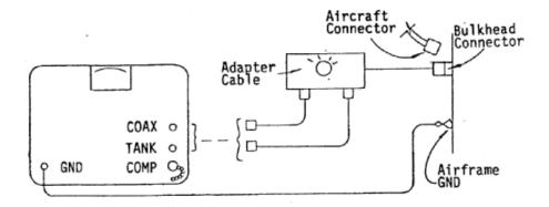
Figure 12 INDIVIDUAL TANK UNIT CAPACITANCE TEST, CONFIGURATION #2
