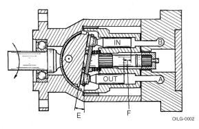
Figure 4. Position B/2, Pump During One Half Delivery From Port B
