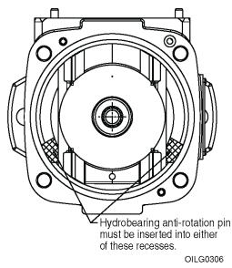
Figure 9. B-Frame and C-Frame Orientation of Pins
