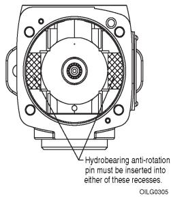
Figure 8. A-Frame Orientation of Pins
