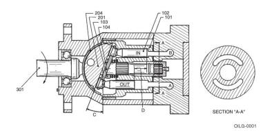
Figure 3. Position B, Pump During Full Delivery From Port B
