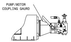
FIGURE 6.4.1 Pump/Motor Coupling Access
