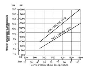
Raise compensator from minimum to maximum outlet pressure. At each condition, increase the outlet pressure until the pump fully de-strokes. At no time should the outlet pressure vary over 150 psi, 10,3 bar from the compensator setting. The control should be steady and stable at all conditions.
