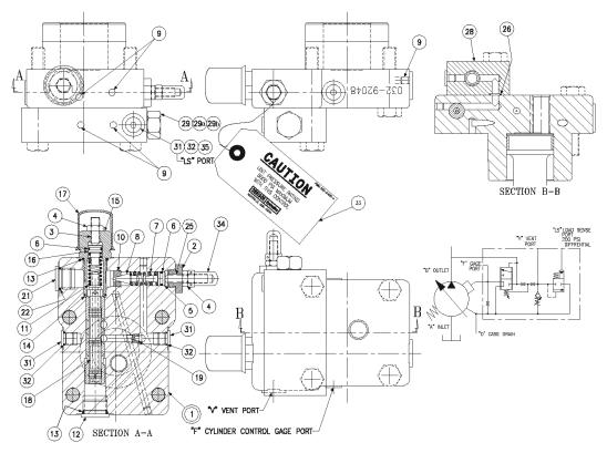
Ref. Figure 12 load sensing compensator control
