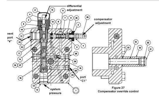
PARTS LIST FOR FIGURE 27 compensator override control P07 compensator override S22-16205 P110 comp. override S22-16206
