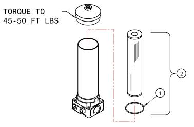
Parts List Fluid Type: Aviation Phosphate Ester, Type IV, V
