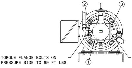
TORQUE FLANGE BOLTS ON INLET SIDE TO 85 FT LBS
