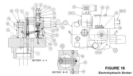
PARTS LIST FOR FIGURE 18 P07 electrohydraulic stroker S22-16204 P110 electrohydraulic stroker S22-16203
