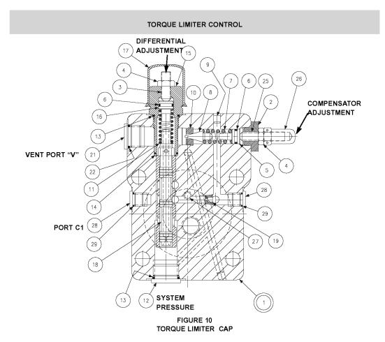
PARTS LIST FOR FIGURE 10 P07 torque limiter cap S22-15407 P110 torque limiter cap S22-15607
