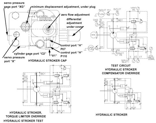
Before testing hydraulic stroker, disable the compensator or torque limiter override, if applicable, by turning the compensator differential adjustment fully in. (See compensator or torque limiter test). **CAUTION:** System must contain a relief valve to limit outlet pressure. Outlet relief valve should be set to minimum pressure.
