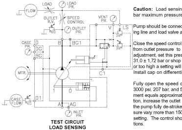
**Caution:** Load sensing control is limited to 5000 psi, 345 bar maximum pressure.
