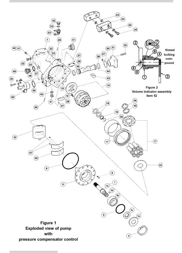
Disassembly Disassemble only as far as necessary to replace or repair worn parts.
