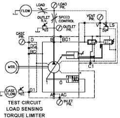
Start prime mover with outlet relief set at 500 psi, 34,5 bar. Apply a load to the pump.
