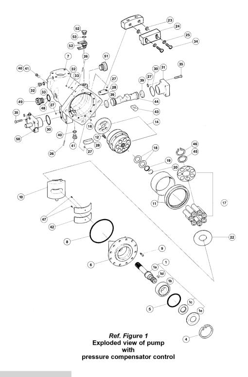
4. Press bearing outer race (11) into housing (7).
