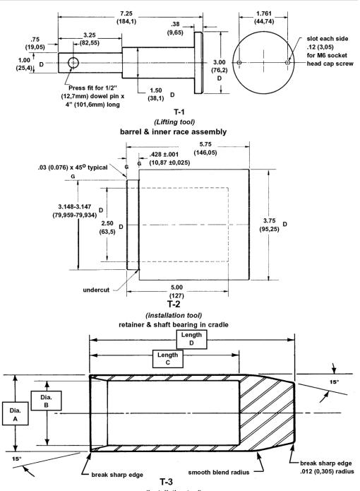
*(installation tool)* shaft seal over shaft
