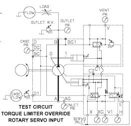
If the pump contains a servo, hydraulic or electrohydraulic stroker control, test that control first (pg. 64, 68 or 69) then set the control to give full displacement on the pump. **CAUTION:** System must contain a relief valve to limit outlet pressure. Outlet relief valve should be set at 500 psi, 34,5 bar.
