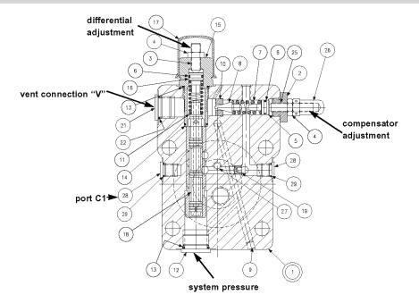
Ref. Figure 14 Load Sensing Torque limiter cap
