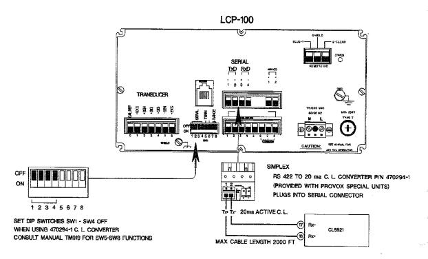
Figure 10-4. Fisher Provox Rear Panel Connections
