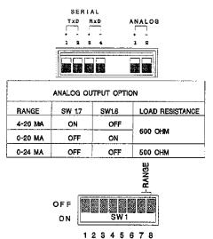
Figure 2-9. Analog Current Selection/Connection
