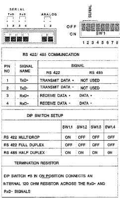
Figure 2-8. Serial Communication Configuration
