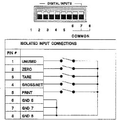
Figure 2-10. Remote Digital Inputs
