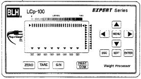
Figure 1-2. The LCp-100 Front Panel
