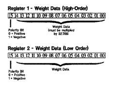
**NOTE**: If a decimal point is required the resulting value must be multiplied by the appropriate fraction, i.e., 0.01 for hundreds of a unit. In the case of mv/V values the multiplier is 0.000001. The LCp-100 range is (-999999/+9999999).
