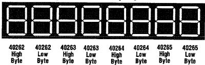
Figure 10-3. Display Write, Register and Byte Allocations
