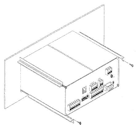
Figure 2-2. Panel Mounting Arrangement
