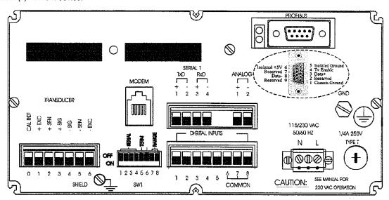
Figure 11-1. Profibus Rear Panel Connections
