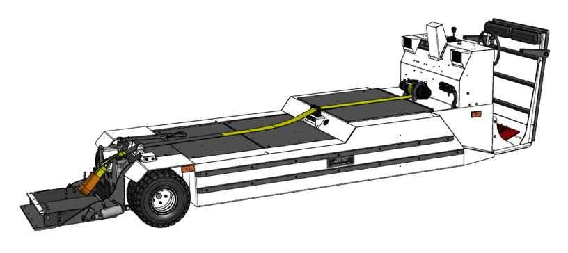
AP8750CX-AL FEATURES: Vehicle Drive: 33.1 HP/24.8 kW, 72 VDC Traction Motor mated with Auburn/Dana 44 Differential. Limited Slip Differential, optional. Motor Speed Control: EV100ZX SCR with On-Board Diagnostics.
