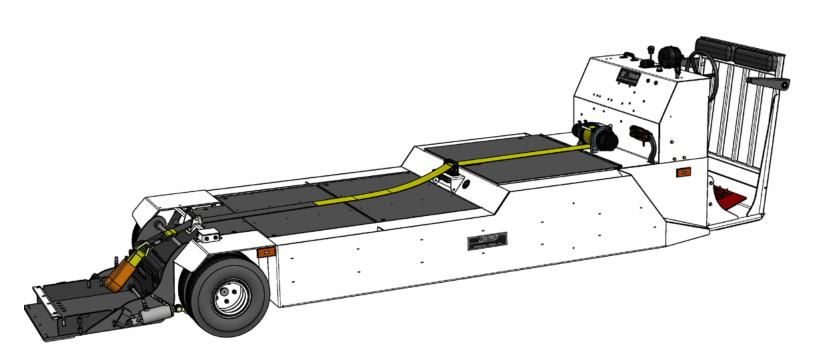
AP8750CX-EZ FEATURES: Vehicle Drive: 33.1 HP/24.8 kW, 72 VDC Traction Motor mated with Auburn/Dana 44 Differential. Limited Slip Differential, optional.
