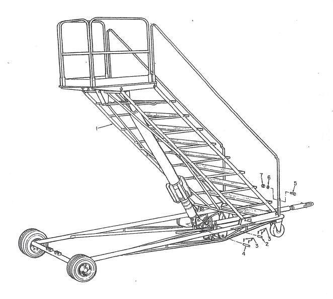
Figure 1. Aircraft Maintenance Platform (Sheet 1 of 5)
