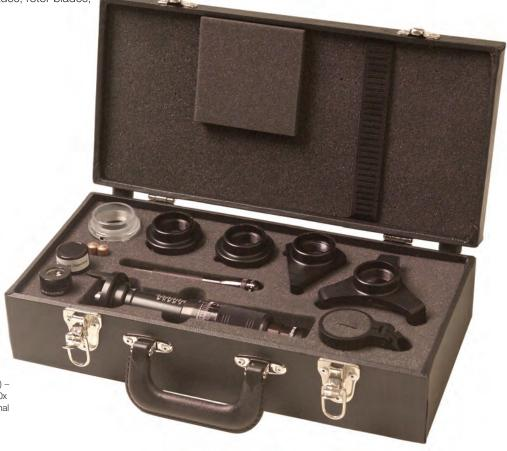
\*Shown: Optical Micrometer Kit (Model 966A1) – Includes 5x and 10x interchangeable optics, 20x eyepiece cell, reticle eyepiece cell; five additional bases, micrometer light, adjustable light bracket and case.
