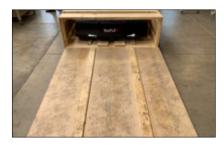
Then pull the two eStops and start the unit. Wait until the unit has booted and the connection has been established. Then you can drive the tug very carefully and as slowly as possible over the ramp.
