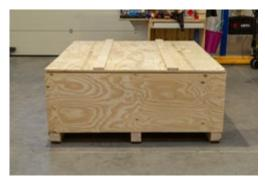
To remove the cover, all bolts on the sides and on top must be loosened. All bolts should be marked with a red dot.
