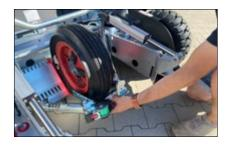
When the strap is released, press the button for automatic capturing and releasing on the remote control. The mount will then begin to lower. Press this button until the nose wheel is on the ground and the arms of the cradle are fully open. The system stops automatically when the end position is reached.
