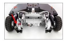
First open the wheel mount using the remote control so that the arms are in the outermost position. Move the tug carefully and slowly towards the nose wheel so that the tug is as centered as possible. Depending on the wheel type (twin or single), first remove the nosewheel spacers (lateral limiters for the nose wheel). These are only required for single-no-sewheel configurations.
