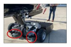
Afterwards the capturing process can be started via the remote control. To do this, press the dedicated button. The mount then automatically moves to the top position, as long as to button remains pressed.
