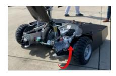
The mount stops automatically in the uppermost position. In order to ensure the best possible safety, the arms must then be secured with the strap attached to the left arm.
