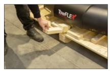
Take the top cover and attach it to the front of the transport box to use it as ramp for the tug.
