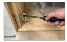
To prevent unwanted movement during transport, there is a wooden wedge in front of the castor wheels, which is bolted to the floor of the box. Remove these bolts and pull out the wedge.
