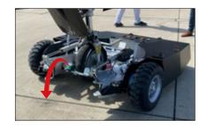
After that, the nose wheel should be cleared and the tug can be moved away from the nosegear carefully.
