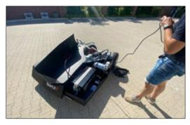
Battery Charging Cable located under the left lid.
