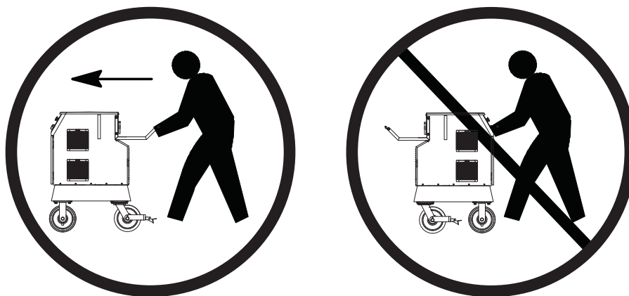
Figure 2. Proper Handling of Ground Power Unit
