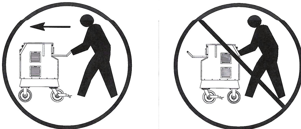
Figure 2. Proper Handling of Ground Power Unit
