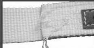
BROKEN OR WORN STITCHES
