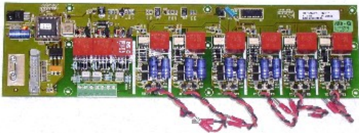
Thyristor/ Gate drive
